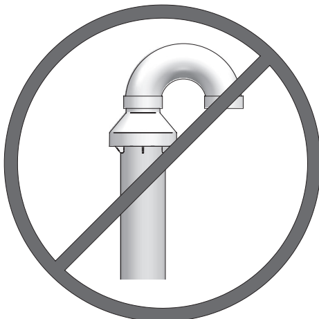
Figure 5-5 Do Not Install U-Bend to Rain Cap
